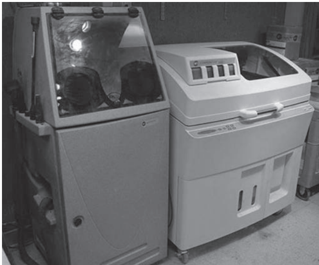
Figure 9. ZPrinter@510- device used for the fabrication of the model (Source: authors)
