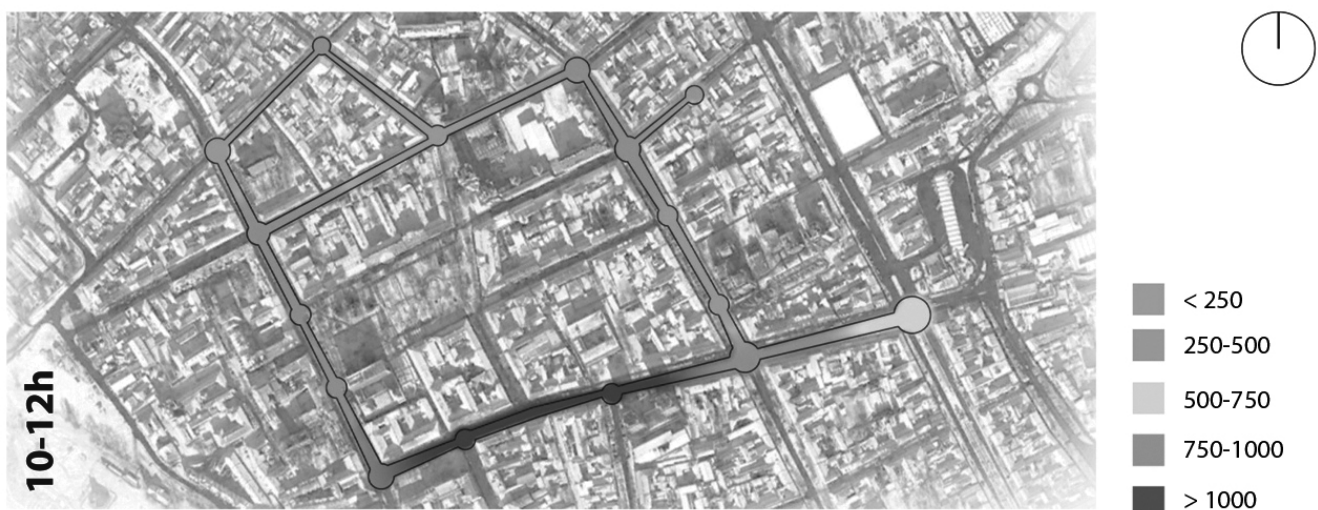
Figure 8: Pančevo. Results of analyses using the Space Syntax method. Source: Aleksandra Đukić, Milena Vukmirović
