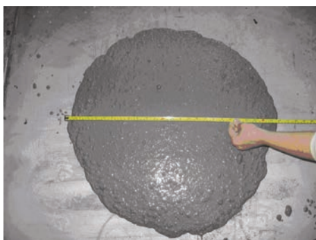
Figure 7: Resulting concrete spread 670 mm (class SF2)
