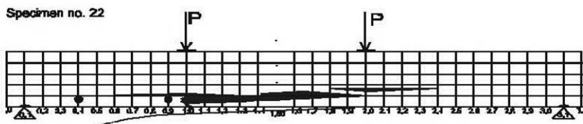
Figure 8. Cracking and crushing of timber fibres in the sample no. 22
